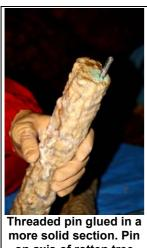
Threaded pin glued in a more solid section. Pin on axis of rotten tree root. Photo by Sonia Taylor-Smith.
